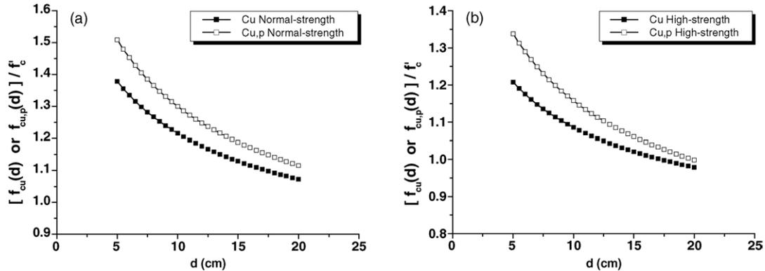
Fig. 6. Effect of placement direction on compressive strength of cubes: (a) normal-strength concrete; (b) high-strength concrete.
