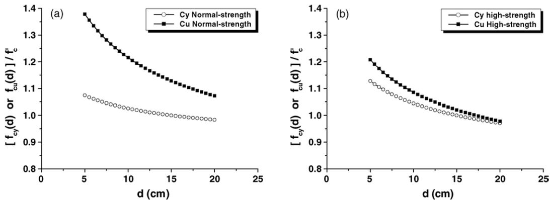
Fig. 8. Effect of strength level on shape effect of compressive strength: (a) normal-strength concrete; (b) high-strength concrete.
