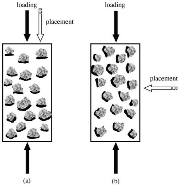
Fig. 4. Illustrations of loading and placement directions.
