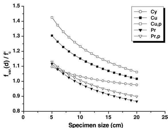
Fig. 9. Relationship between relative strengths and specimen size  $d$ .
