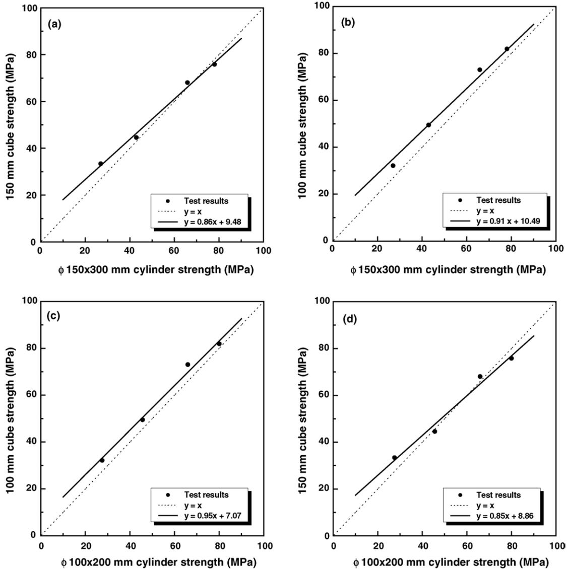
Fig. 10. (a) Relationship between compressive strengths of 150 mm cube and  $\phi 150 \text{ mm} \times 300 \text{ mm}$  cylinder; (b) relationship between compressive strengths of 100 mm cube and  $\phi 150 \text{ mm} \times 300 \text{ mm}$  cylinder; (c) relationship between compressive strengths of 100 mm cube and  $\phi 100 \text{ mm} \times 200 \text{ mm}$  cylinder; (d) relationship between compressive strengths of 150 mm cube and  $\phi 100 \text{ mm} \times 200 \text{ mm}$  cylinder.
