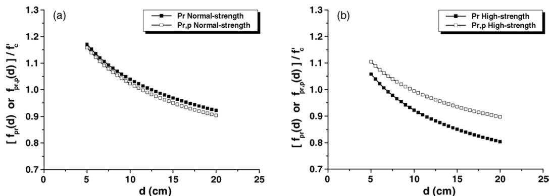
Fig. 7. Effect of placement direction on compressive strength of prisms: (a) normal-strength concrete; (b) high-strength concrete.
