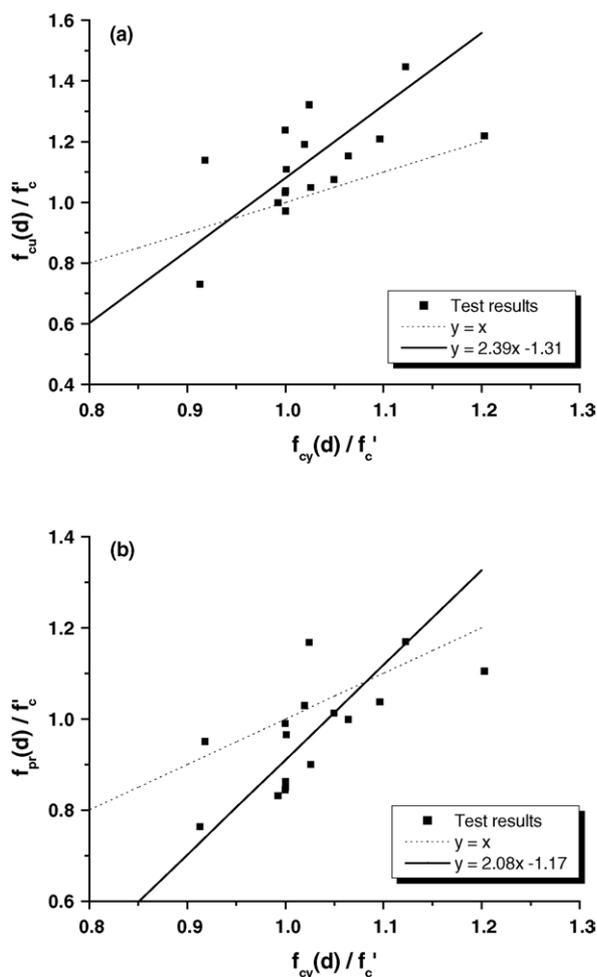
Fig. 11. Generalization of strength prediction equations for cubes and prisms: (a) relationship between strengths of cube and cylinder; (b) relationship between strengths of prism and cylinder.
