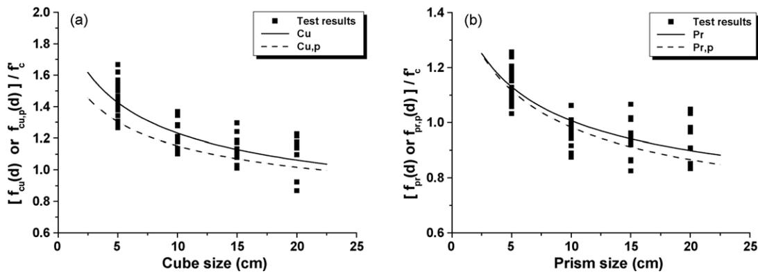
Fig. 5. Size effect with placement direction: (a) cubes; (b) prisms.
