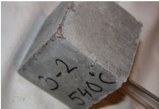
Figure 3: FRC with carbon/steel at 540 °C
