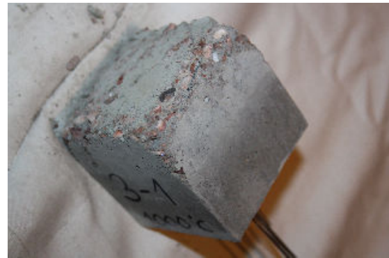
Figure 4: FRC with carbon/steel at 1000 °C
