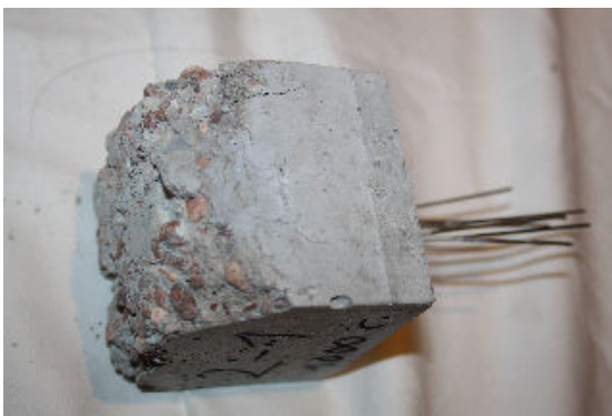
Figure 5: FRC with PP/steel under 1000 °C
