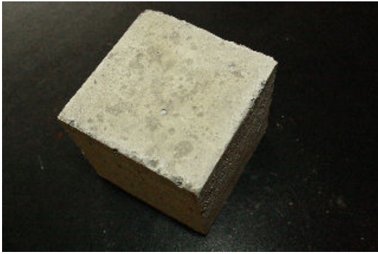
Figure 1: FRC with carbon/steel without heating
