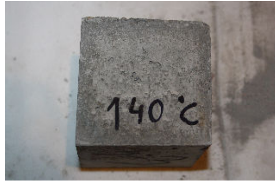
Figure 2: FRC with carbon/steel under 140 °C
