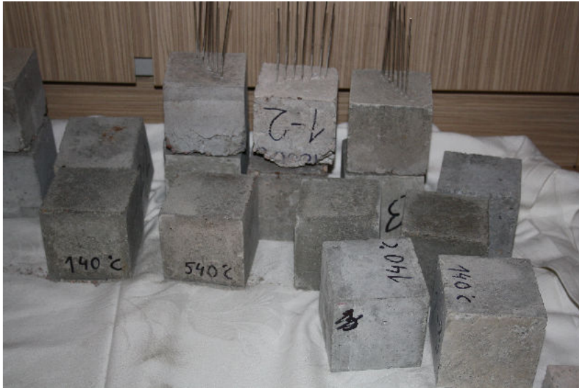
Figure 7: All samples from the experiments including thermocouples
