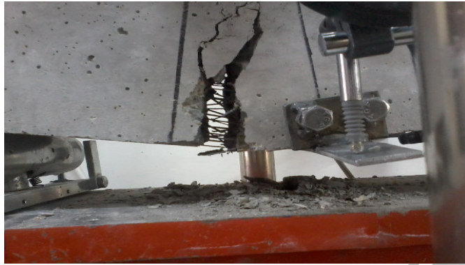
Figure 3. Fibers bridging at crack section
