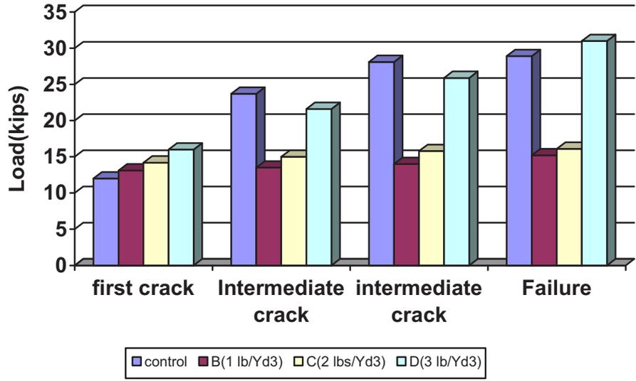
**Figure 11: Effect of Fibers on Shear strength of RCC beams (Set-2)**
