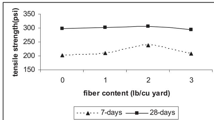
**Figure 7: Effect of Fibers on Flexural strength of plain concrete beams**
