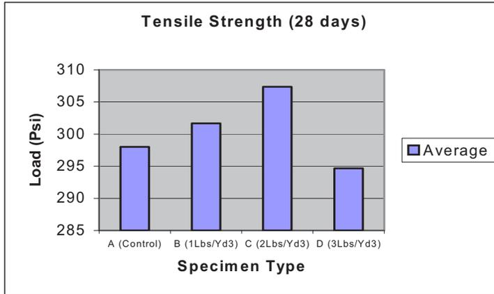
**Figure 6: Comparison of Tensile strength at 7 and 28 days**
