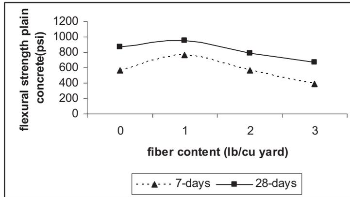
**Figure 8: Effect of Fibers on Flexural strength of RCC beams**
