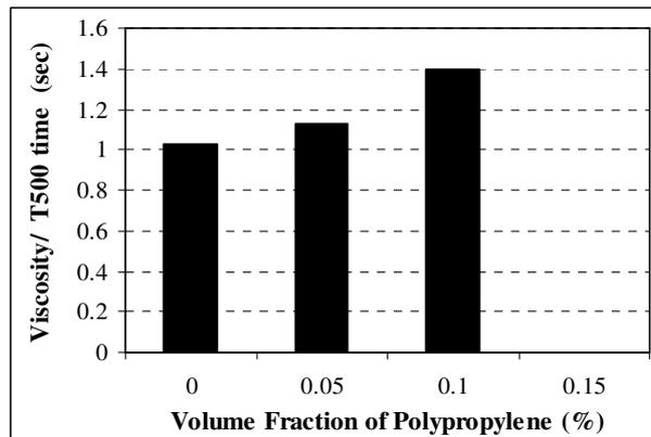
**Figure 2:** Effect of Polypropylene Fiber Addition on the Viscosity of SCC Mixes
