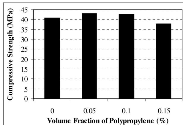
**Figure 5:** Effect of Polypropylene Fiber Addition on the Compressive Strength of SCC
