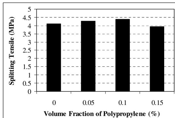
**Figure 6:** Effect of Polypropylene Fiber Addition on the Splitting Tensile Strength of SCC
