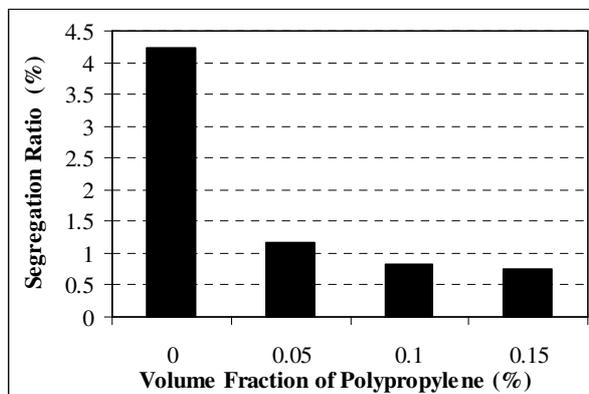
**Figure 4:** Effect of Polypropylene Fiber Addition on Segregation Ratio of SCC Mixes
