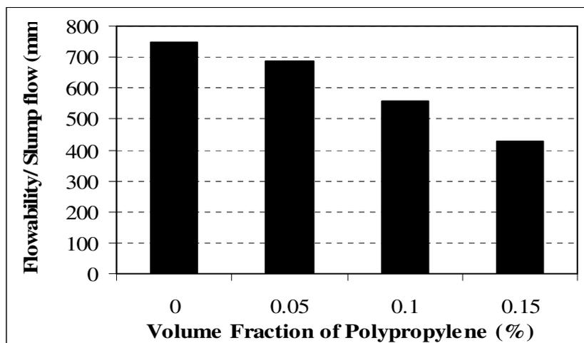
**Figure 1:** Effect of Polypropylene Fiber Addition on the Flowability of SCC Mixes
