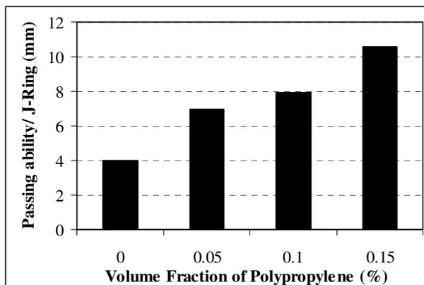
**Figure 3:** Effect of Polypropylene Fiber Addition on the Passing Ability of SCC Mixes
