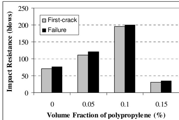
**Figure 7:** Effect of Polypropylene Fiber Addition on the Impact Resistance of SCC;
