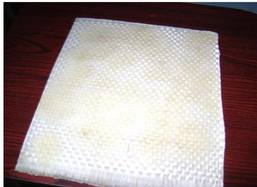
Fig. 2. GFRTP Composite Laminate
