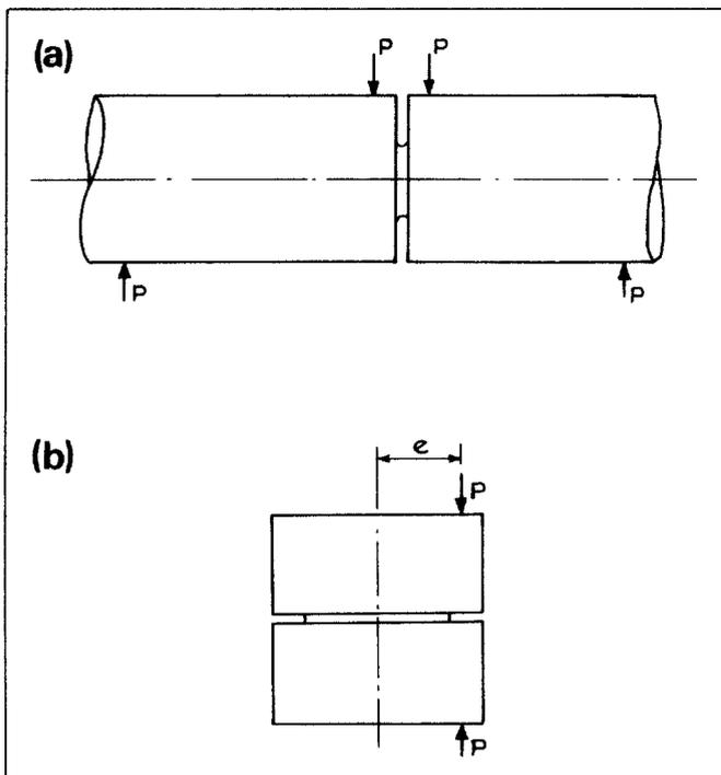
Figure 1 Circumferentially notched round bar test specimens. (a) Test specimen subjected to four-point bending (b) Test specimen subjected to eccentric loading
