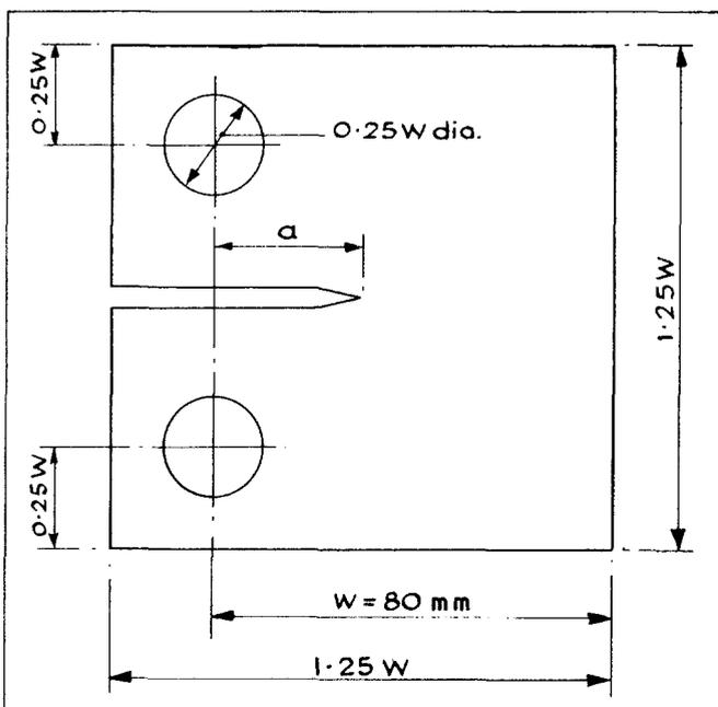
Figure 3 Compact tension specimen details
