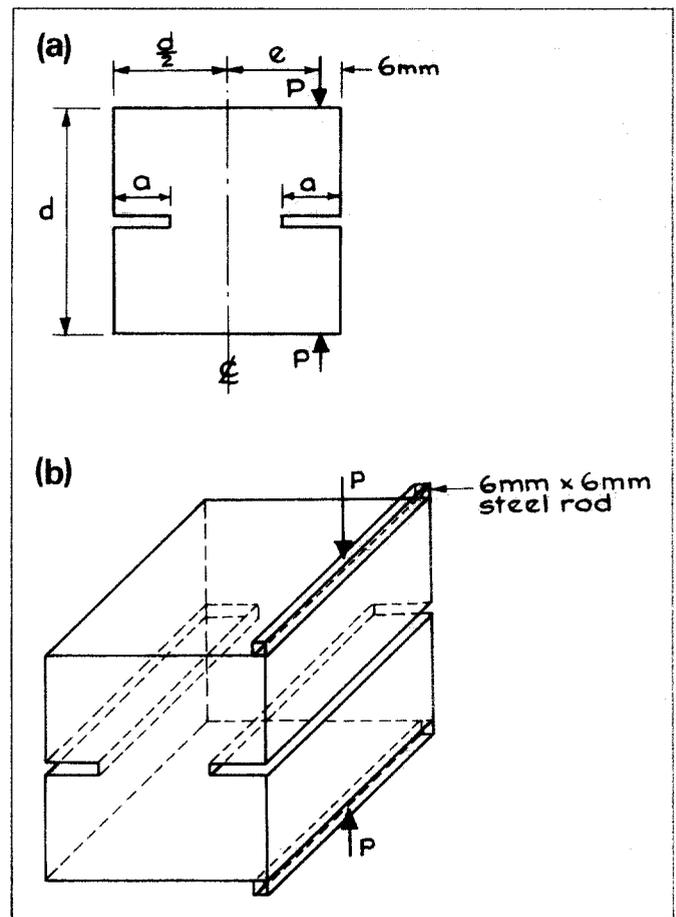
Figure 2 Geometry and loading details of test specimen. (a) Geometrical details of split-cube (b) Loading arrangement for split-cube
