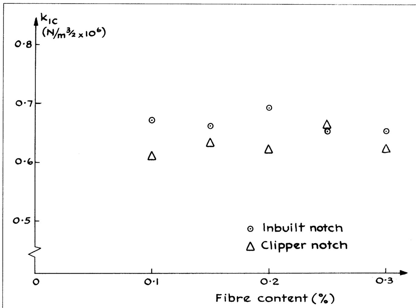
Figure 5 Variation of fracture toughness for CTS specimens
