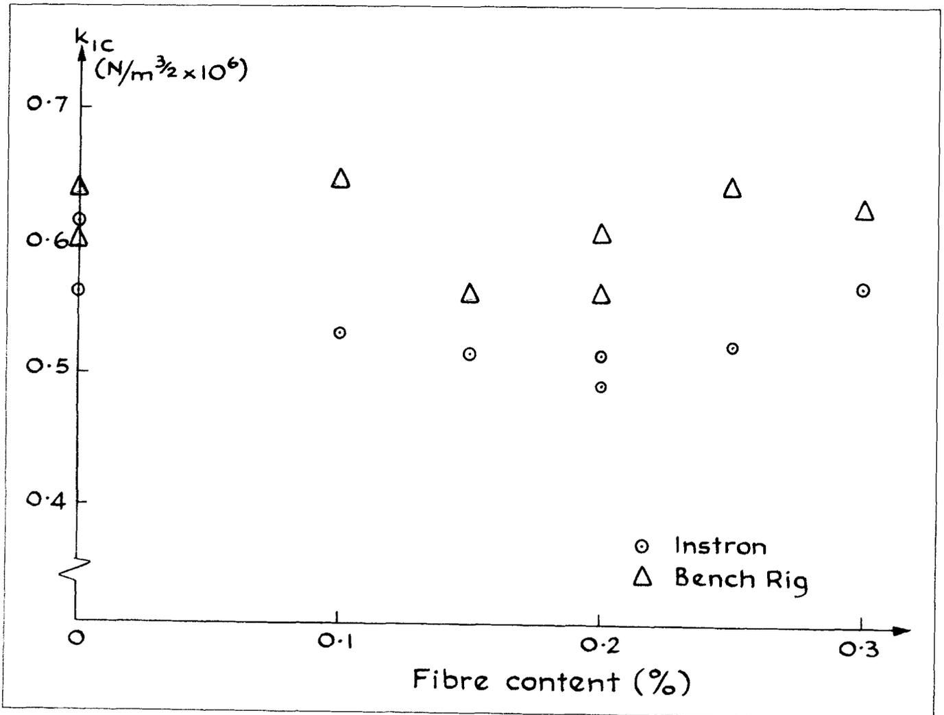
Figure 4 Variation of fracture toughness with fibre content
