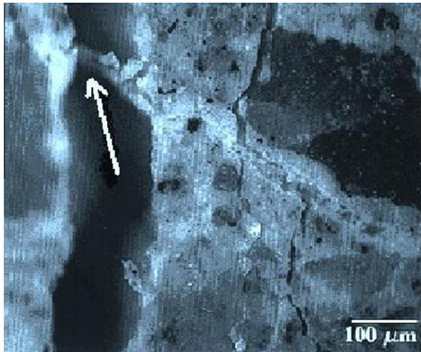
Fig. 4. Microscopic picture of the intersections of fiber and crack formed on the concrete surface.
