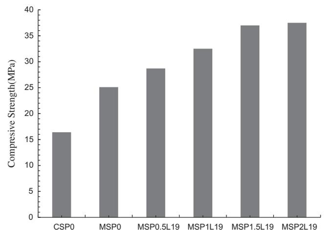
Fig. 3. Compressive strength of different concrete samples after 28 days curing.
