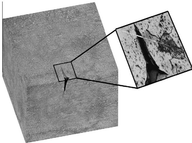
Fig. 5. graphical schematic of the prevention of the crack propagation by forming connection bridge by fiber.
