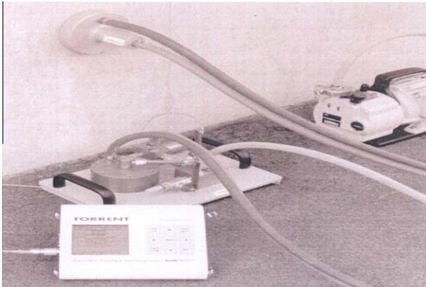
Fig. 1. Torrent system for permeability measurement.
