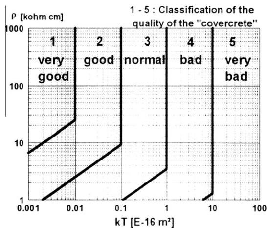
Fig. 2. Determination of concrete quality based on the permeability and strength [18].
