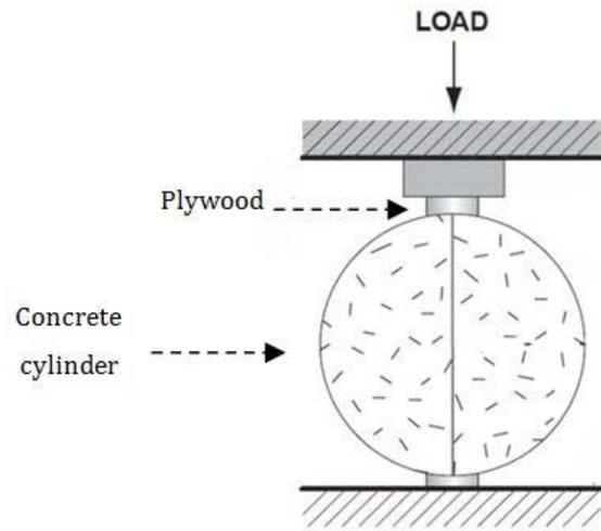
FIGURE 3. Schematic of split tensile strength test.
