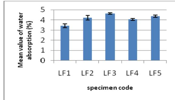
FIGURE 4. Water absorption of LWC specimens.
