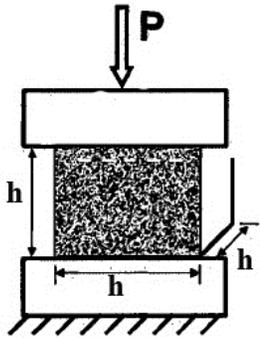
FIGURE 2. Schematic of compressive strength test.
